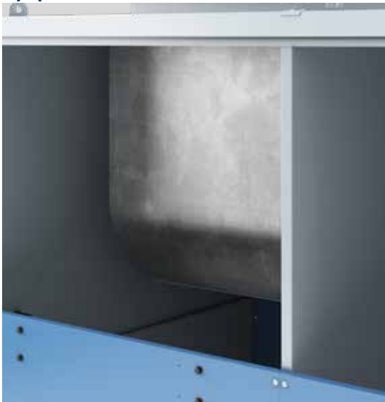
Internal panel to avoid the by-pass effect
